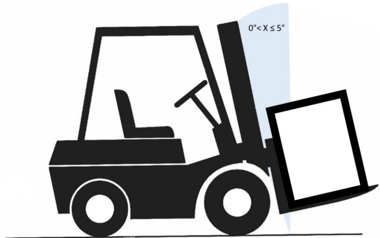
Fig. 9: Tilt angle for transporting with a forklift truck
